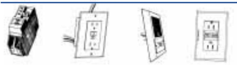
Three-pronged plugs and outlets, and polarized plugs and outlets offer enhanced protection against potential shock when provided on specific products. These measures should never be circumvented by sawing or breaking off the third prong or attempting to widen an outlet slot.
